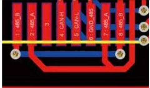
Definition of RJ45 Port Pin for Meter-485
