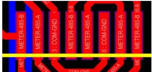
Definition of RJ45 Port Pin of "Modbus port" for remotely monitoring
