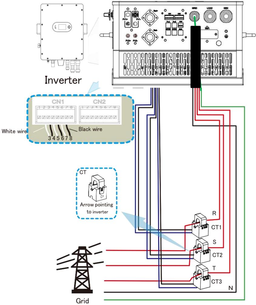
**\*Note:** when the reading of the load power on the LCD is not correct, please reverse the CT arrow.
