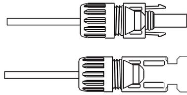
Pic 3.5 connector with cap nut screwed on
