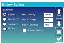
**Battery capacity:** it tells Deye hybrid inverter to know your battery bank size.
