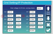
**Normal connect**: The allowed grid voltage/frequency range when the inverter first time connect to the grid. **Normal Ramp rate**: It is the startup power ramp.
