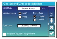
Grid Mode:General Standard, UL1741 & IEEE1547, CPUC RULE21, SRD-UL-1741, CEI 0-21, Australia A, Australia B, Australia C, EN50549\_CZ-PPDS(>16A), NewZealand, VDE4105, OVE-Directive R25. Please follow the local grid code and then choose the corresponding grid standard. Grid level: there're several voltage levels for the inverter output voltage when it is in off-grid mode. LN:230VAC LL:400VAC, LN:240VAC LL:420VAC, LN:120VAC LL:208VAC, LN:133VAC LL:230VAC.
