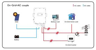
The 1st priority power of the system is always the PV power, then 2nd and 3rd priority power will be the battery bank or grid according to the settings. The last power backup will be the Generator if it is available.
