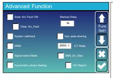
Solar Arc Fault ON: This is only for US. System selfcheck: Disable. this is only for factory. Gen Peak-shaving: Enable When the power of the generator exceeds the rated value of it, the inverter will provide the redundant part to ensure that the generator will not overload.
