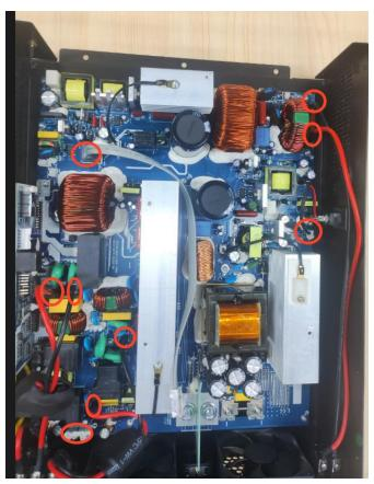
(9) Remove 2 screws as below; Then take out the control board
