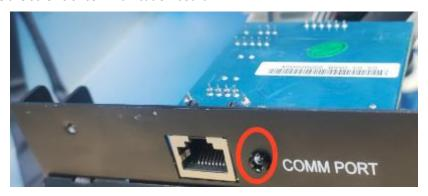
(5) Remove the antenna, Then take out the communication board.
