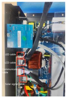
4 Remove the screws of communication board
