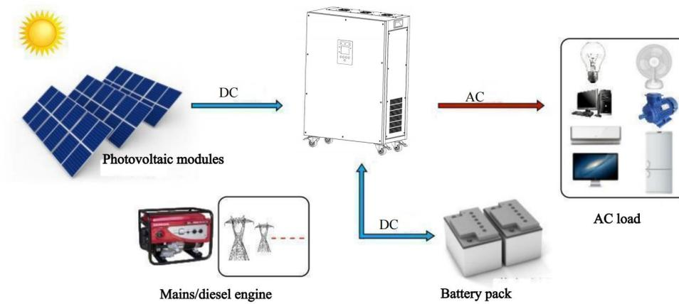
(3) In the mains priority mode, when the photovoltaic panel does not generate power at night or on a cloudy or rainy day and the mains input is normal, the system works as shown in the figure below:
