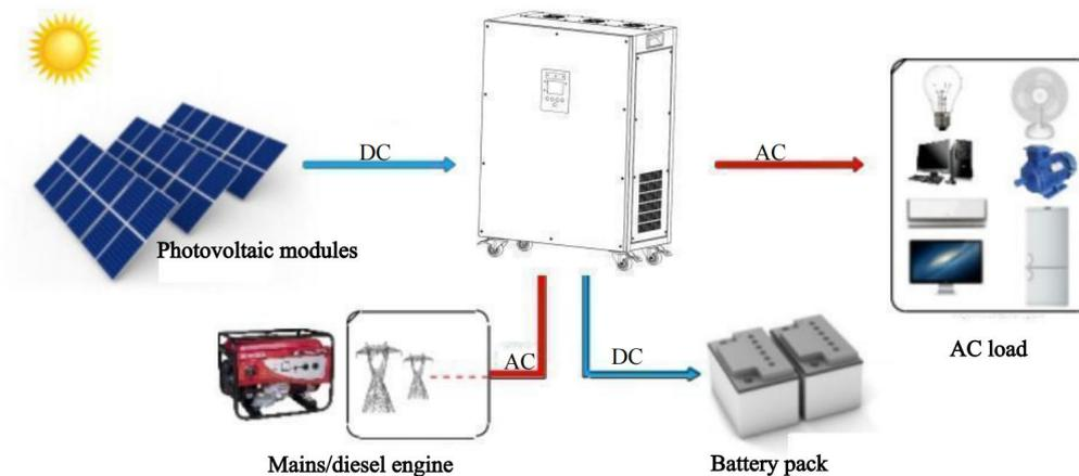
(2) In the mains priority mode, when the photovoltaic panel generates electricity with sufficient sunlight and the mains input is abnormal, the system works as shown in the figure below:
