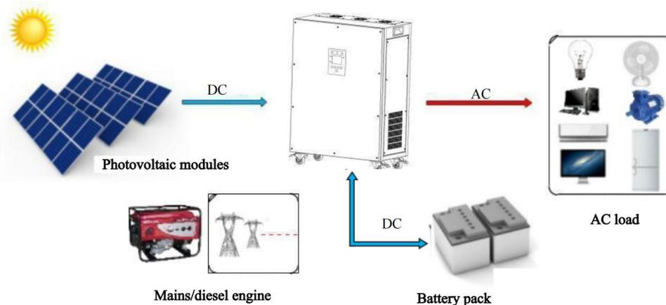
(2) In battery priority mode, when the photovoltaic panel does not generate electricity at night or on a cloudy or rainy day and the battery voltage is normal, the system works as shown in the figure below:
