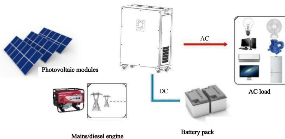
(3) In battery priority mode, when the photovoltaic panel does not generate electricity at night or on a cloudy or rainy day and the battery is low, the system works as shown in the figure below:
