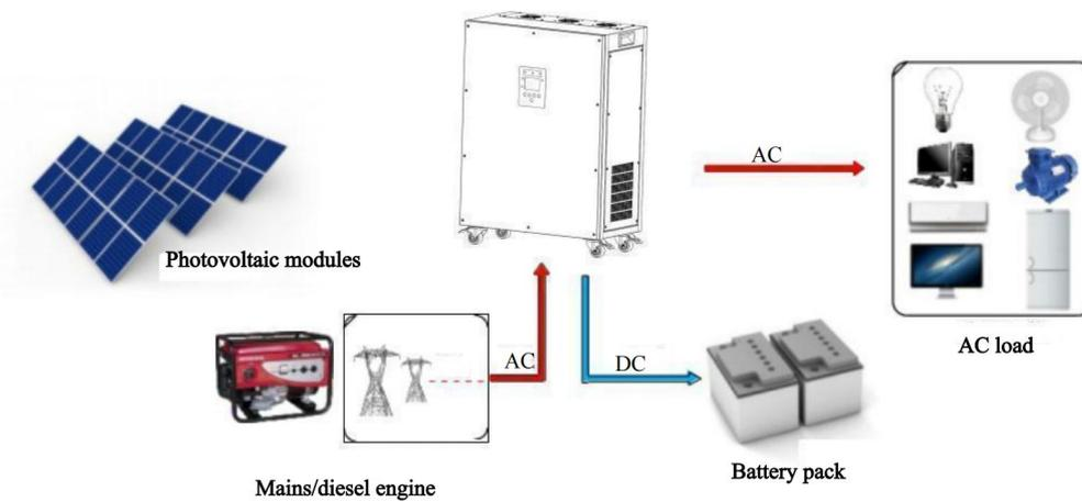
(4) In the mains priority mode, when the photovoltaic panel does not generate electricity at night or on a cloudy or rainy day, the mains input is abnormal and the battery voltage is normal, the system works as shown in the figure below:
