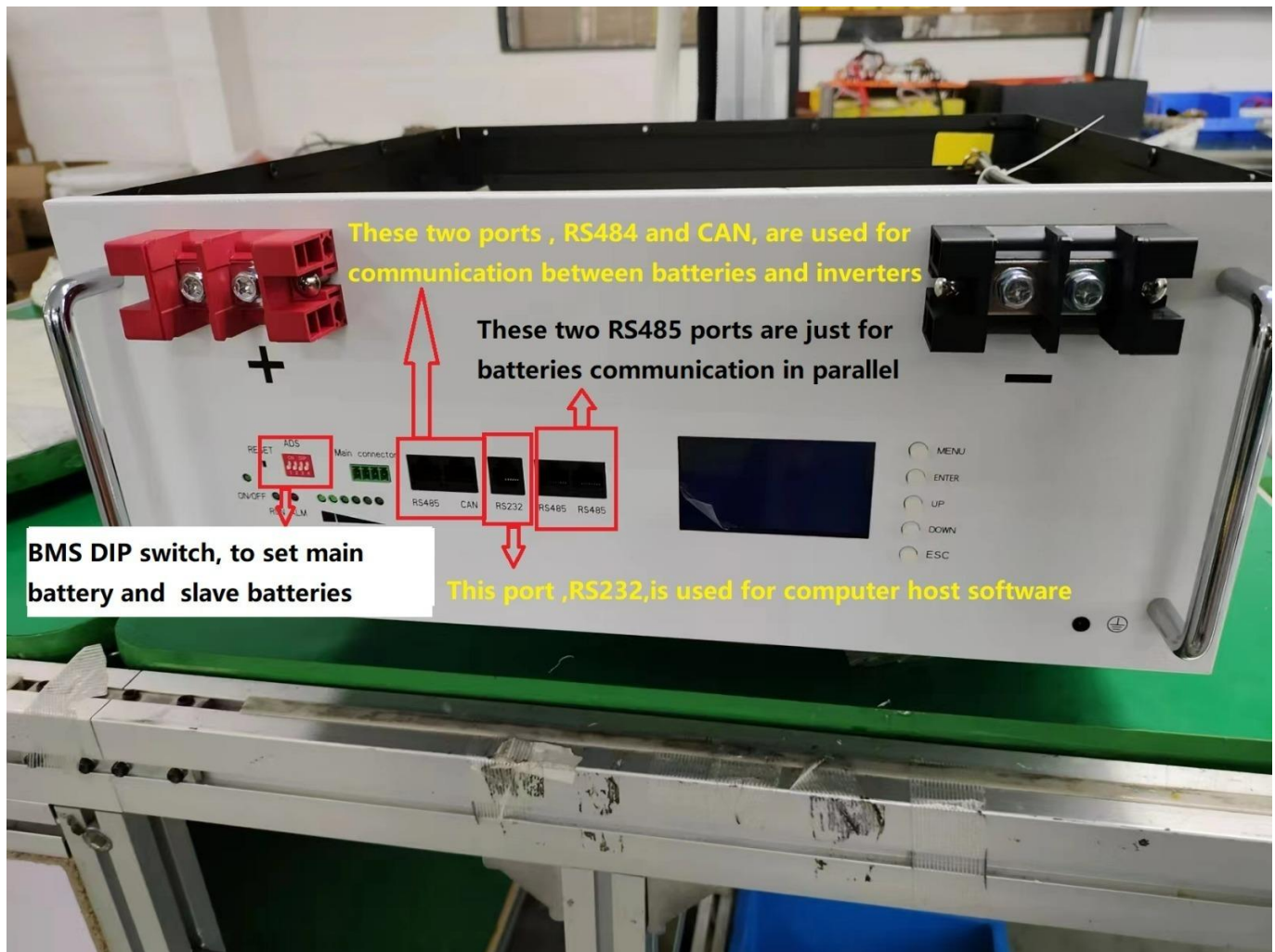
FIG 5: OGM POWERWALL LITHIUM BATTERY PORT/SWITCH FUNCTIONS EXPLAINED.
