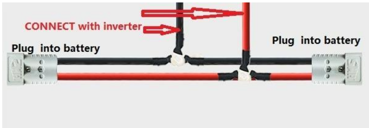
FIG 2: ANDERSEN CABLES SPLICED AND JOINED TO INVERTER LEAD CABLES .
