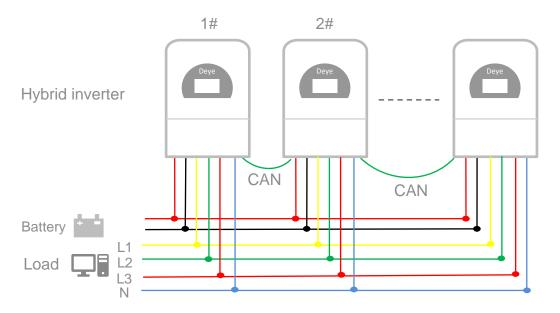
■ The above diagram only shows the load port connection method. The grid port connection method is same with load port connection method.
