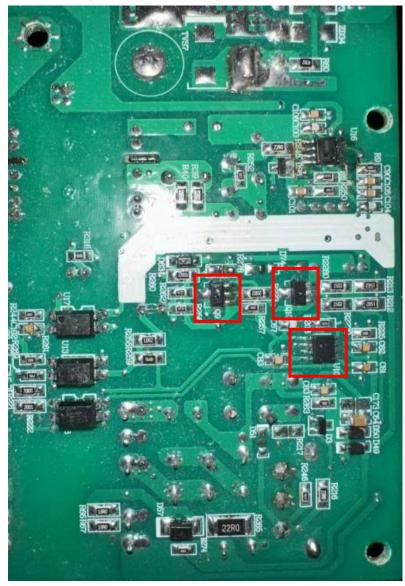
If abnormal, check whether the components here are damaged.
