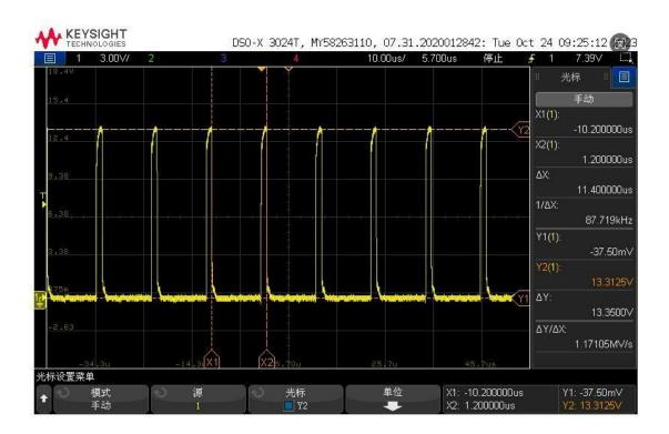
Pin 3 is the current protection waveform. The amplitude cannot exceed 1V when measured by an oscilloscope.
