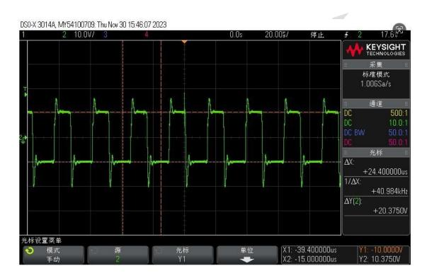
The reference amplitude of Q30 driving waveform is about 10.5V and the frequency is about 40KHz
