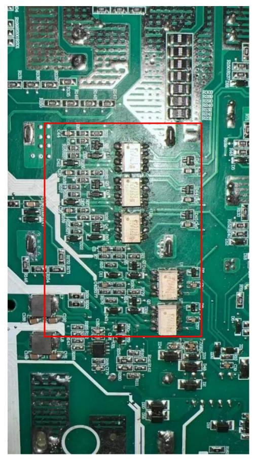
, If it does not return to normal , it is judged as a BUS voltage detection failure .
