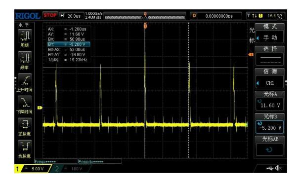
The reference amplitude of D1 waveform is about -384V and the frequency is 19.23KHz
