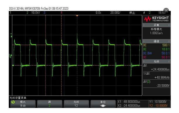
The reference amplitude of Q28 driving waveform is about 10.5V and the frequency is about 40KHz
