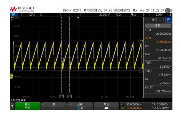
The voltage of pin 6 is about 3.6V
