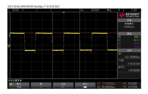
The reference amplitude of the inverter drive waveform of the QA1 power frequency arm is about 15V and the frequency is 50Hz
