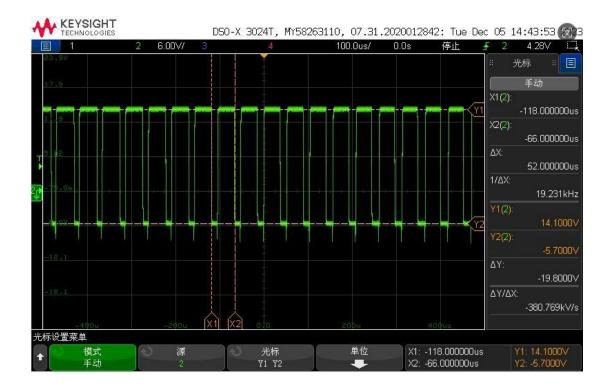
The reference amplitude of the inverter drive waveform of the QC1 power frequency arm is about 15V and the frequency is 50Hz
