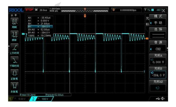
The D24 waveform reference amplitude is approximately -382V and the frequency is 19.23KHz
