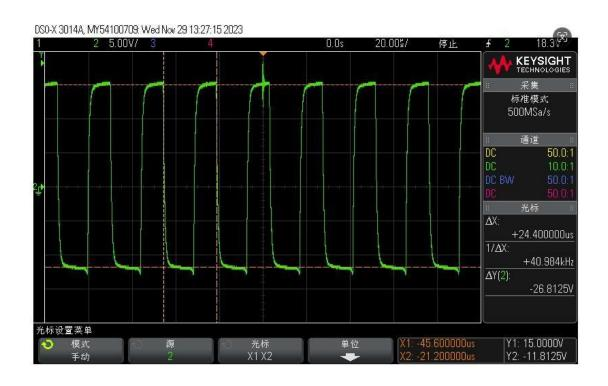
The reference amplitude of Q40 driving waveform is about 15V and the frequency is  $40\mbox{KHz}$
