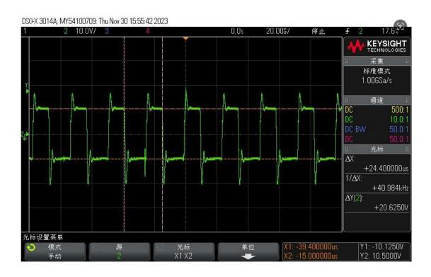
The reference amplitude of Q29 driving waveform is about 10.5V and the frequency is  $40\mbox{KHz}$
