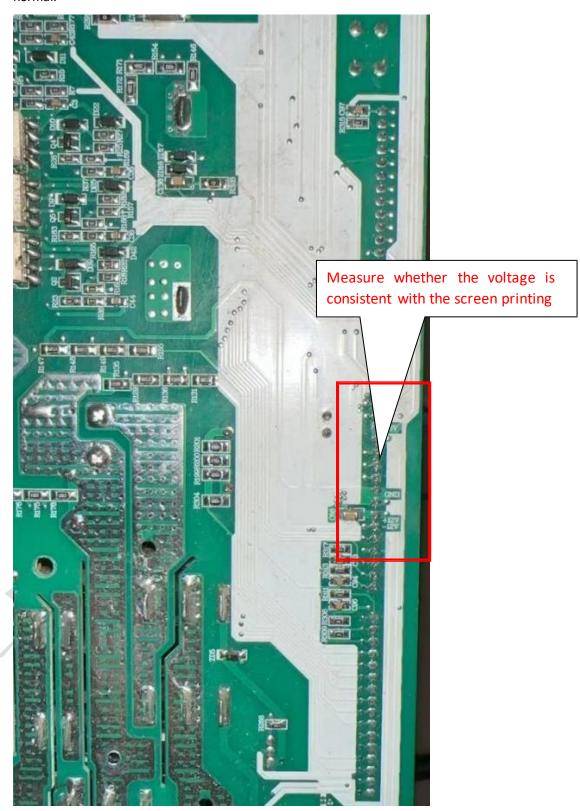
7. If both are normal, check whether the SMD diode D54 and the three-terminal voltage regulator U5 are damaged. If there is no -12V power supply, check whether the SMD diode D70 and the three-terminal voltage regulator U20 are damaged.
