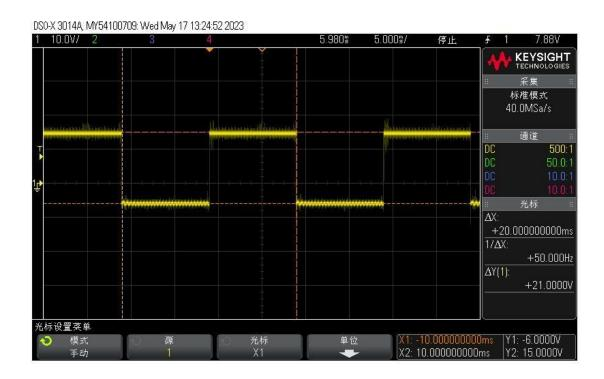
The reference amplitude of the inverter drive waveform of the QD2 power frequency arm is about 14V and the frequency is 19.23KHz
