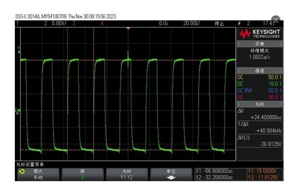
The reference amplitude of Q13 driving frequency is about 15V and the frequency is 40KHz
