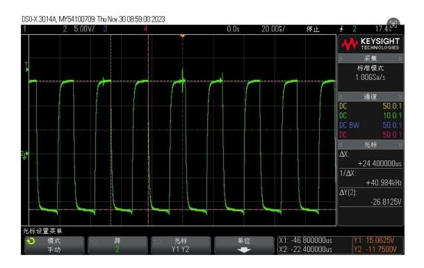
Q24 drive waveform reference amplitude is about 15V frequency 40KHz
