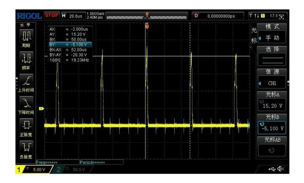
Q5 GS drive waveform reference amplitude is about 11.6V frequency is 19.23KHz
