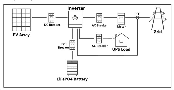
The diagram is the household solar energy storage system. And it is suitable for off-grid and hybrid system.
