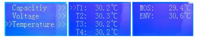
Display 4 cell temperatures, 1 MOS temperature, 1 ambient temperature
