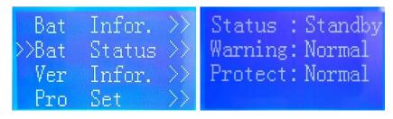
StatusIn-battery state, Standby-Resting state, CHG-On charge, DSG-In discharge state
