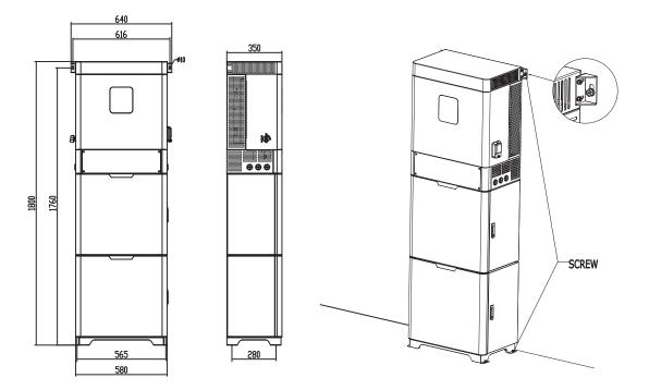
Step 6: The battery fixing, as shown in the figure, push from the right, and a total of 24 M5\*12 screws are used.Please pay attention to the direction when assembling the battery.
