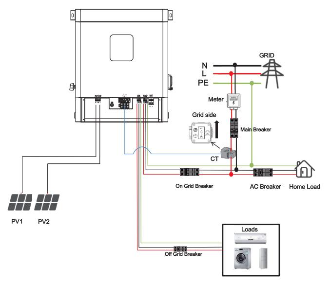
Hybrid inverter are designed for single phase grid. Voltage is 220/230/240V, frequency is 50/60Hz. Other technical requests should comply with the requirement of the local public grid.
