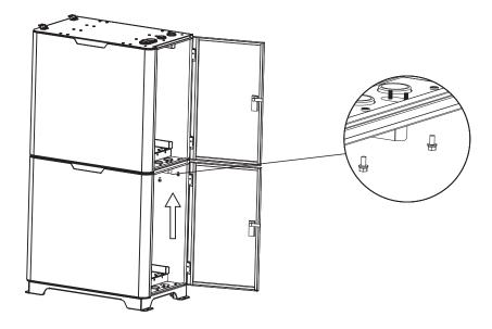
Step 4: PCS is fixed, the method is the same as step 2&step 3. To facilitate pushing to the right, the coil can be removed before assembly.
