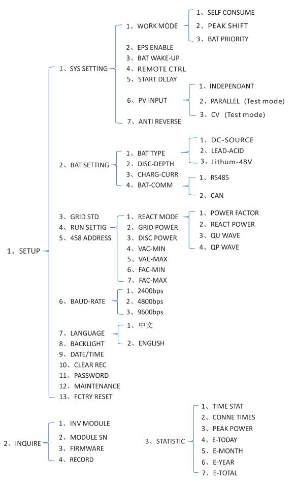
For example,Before selecting the mode, you can set it up ac cording to the local power grid, PV input mode and battery type.
