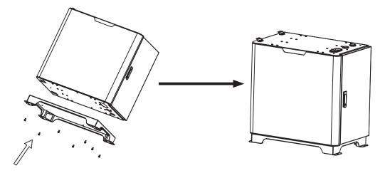
Step 1:Fixing the bottom with the battery box 1, using 8 M5\*12 screws
