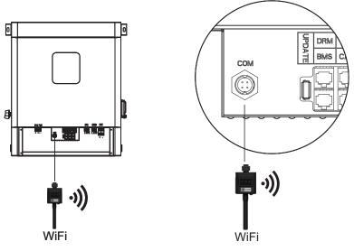
Step1. Plug Wifi into "WiFi" port at the bottom of the inverter.
